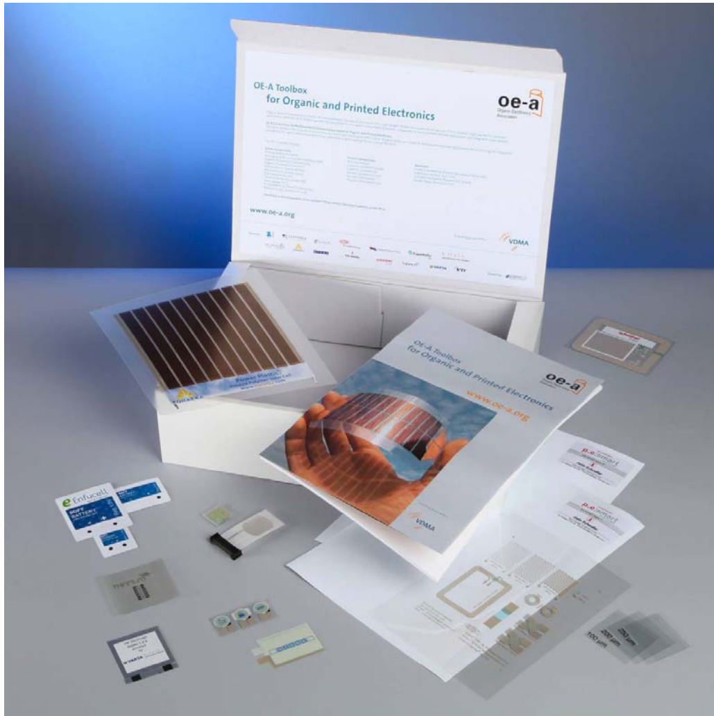
Photo: „OE-A Toolbox“ with more than 20 different components from printed memories to a flexible solar cell (Photo: OE-A).
